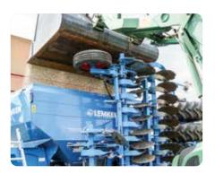
Large fertiliser hopper The generously dimensioned seed hopper in the Compact-Solitair serves as fertiliser tank when using the implement for precision seeding. The maize pack also comprises a metering system that is suitable for fertiliser and an additional hydraulic supply for the single-seed drill. An additional harrow at the coupling frame provides for optimum levelling behind the tyre packer.
