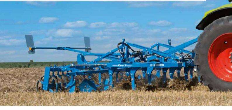
The Karat 9 intensive cultivator is available in working widths of 4 and 5 metres, of which the tines, are arranged on the cultivator frame with an average line distance of about 28 cm to achieve thorough mixing of soil and straw. The symmetrical tine arrangement effectively prevents lateral pull during work.
