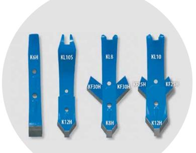
Four soldered carbide plates ensure an extremely long service life of share points. A reinforced carrier material delivers an optimal balance between carbide and steel wear. The smart use of materials on the cones and overlap sections of the share points protects the attachment bolt against wear.
