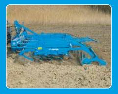
**Favourable centre of gravity** The short and compact design of the System-Korund means that the seed bed combination has a favourable centre of gravity. This means it can be used with tractors with a lower lifting power.
