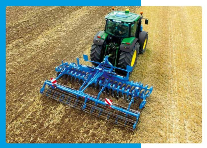
Double rollers consist of two rollers with diameters of 400 mm each or one roller with a diameter of 540 mm and one with a diameter of 400 mm.
