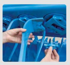
Replacing a quick-change tine
