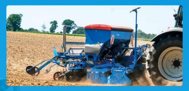
It is becoming ever more important to adjust the intensity of the seedbed preparation to the prevailing field conditions. Practice shows that the power harrow is a very versatile and efficient device and therefore best performs this preparatory task.
